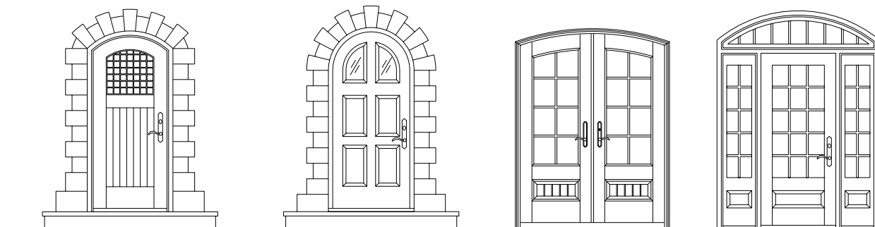
Segmented arched top main entry door with set stone quoin surround
