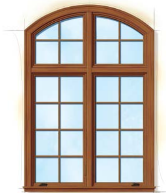
Casement and transom window combination (interior)
