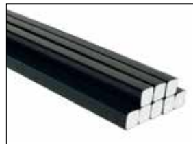
Beveled composite balusters (Available in all colors) 29.5 in. for a 36-in. rail height 35.5 in. for a 42-in. rail height
